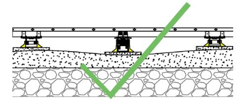
NewTechWood products shown above can be on pedestals or jacks if the surface is uneven. Consult with the pedestal or jack manufacturer before using the product to ensure its compatibility with NewTechWood's products.
