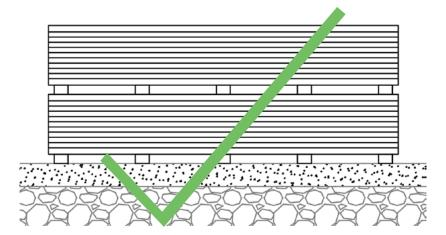
NewTechWood products shown above put on a flat surface on joists, this is the correct way for storage.
