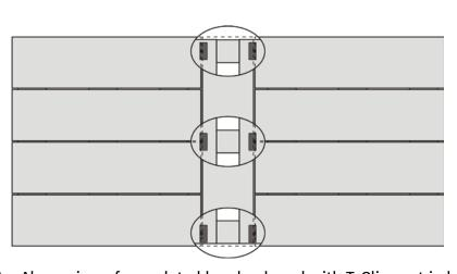
Note: Above view of completed breaker board with T-Clips cut in half.
