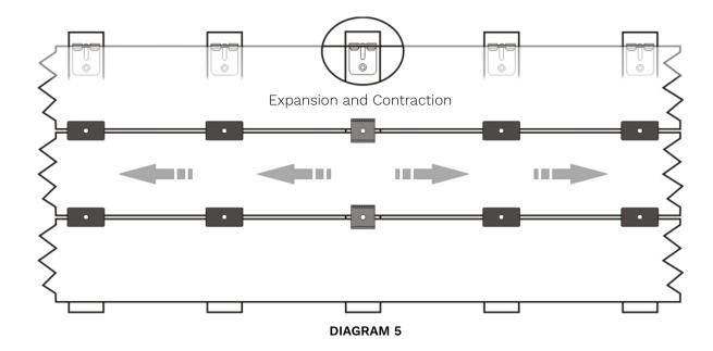
When installing two boards across the deck, locking clips are recommended to be used at the butt joints to ensure proper gapping during expansion and contraction as shown in Diagram 6.
