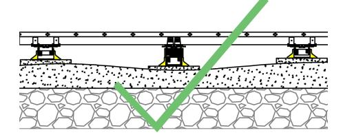
NewTechWood products shown above can be on pedestals or jacks if the surface is uneven. Consult with the pedestal or jack manufacturer before using the product to ensure its compatibility with NewTechWood's products.
