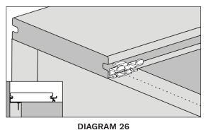
3 Next, screw the clips into the joists at a 45 degree angle as shown in Diagram 27.
